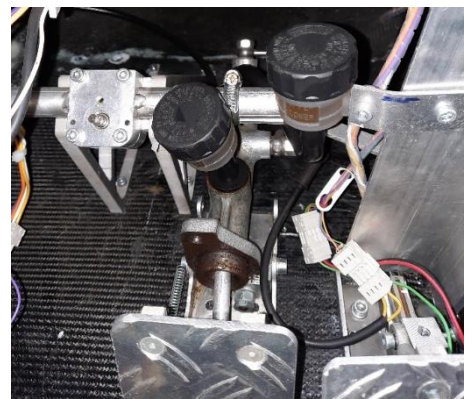
Figure 2: single master two circuit brake cylinder
